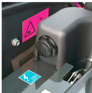
12V external power outlet This power source outlet is a cigarette lighter socket which is the same as that of automobile.
