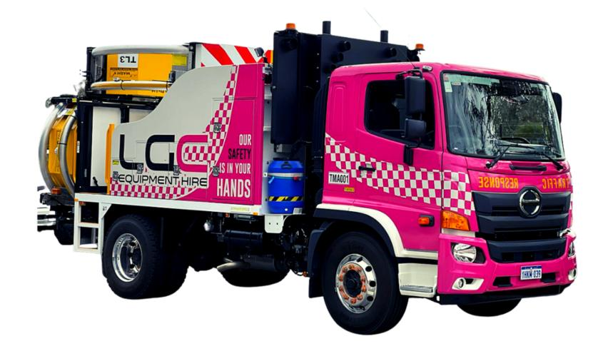
Scorpion II TL-3 TMA - is the world's first MASH Tested, Passed, and Eligible Truck Mounted Attenuator.
