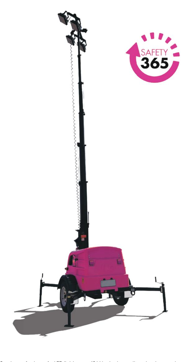
This 9 m tower features 4 x LED lights on a 48 V 'extra low voltage' system and weighs just 1100 kg, enabling easy one person set-up. Designed and manufactured in Australia the Metro-LED tower SLL provides the value you need without sacrificing performance and quality you require.
